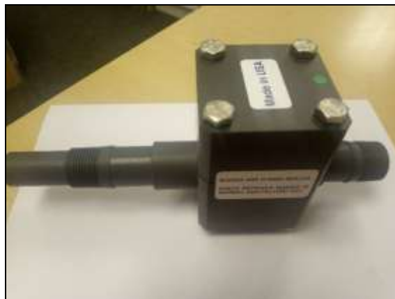
Sample of chlorine gas vacuum injector
